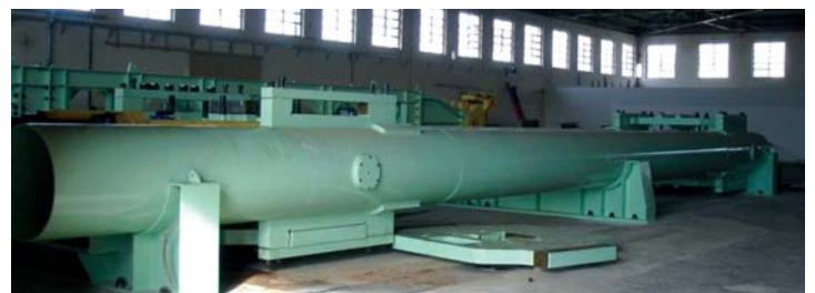
Tension to tension tests
